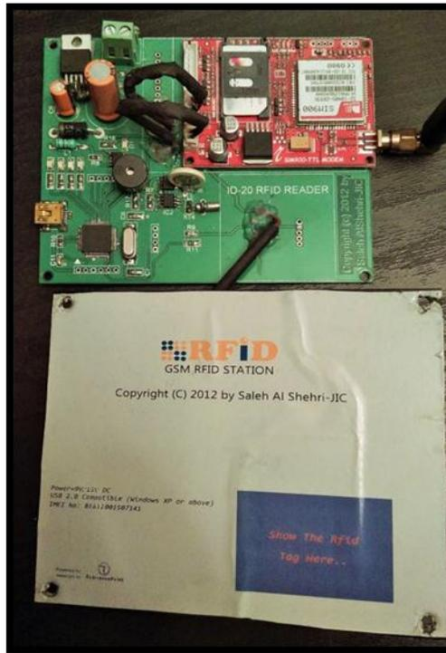
Fig. 2: RFID reader with GSM module.
