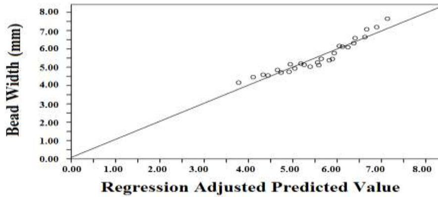
Fig.5. Experimental and predicted values of TIG weld pool for bead width
