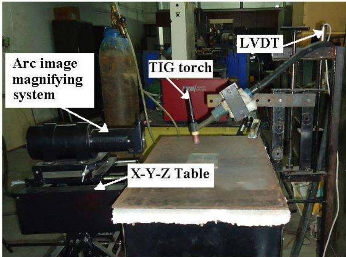
Fig.1 Experimental set-up of TIG welding with arc image magnifying system
