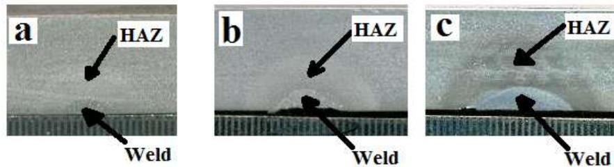
Fig. 4 Macrostructure zones of TIG weld pool geometries
