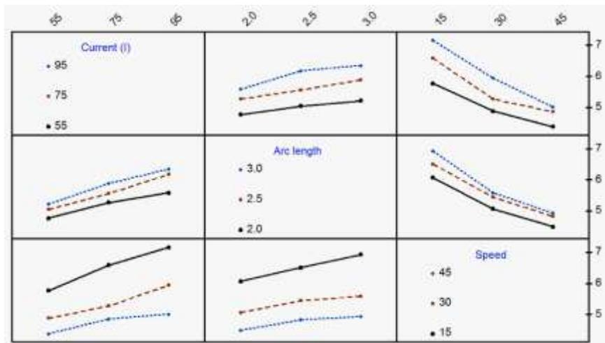
Fig. 6 Interaction plots means for bead width (BW)
