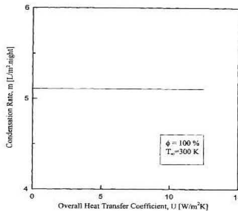
Fig. 5: Effect of heat transfer coefficient on condensation rate
