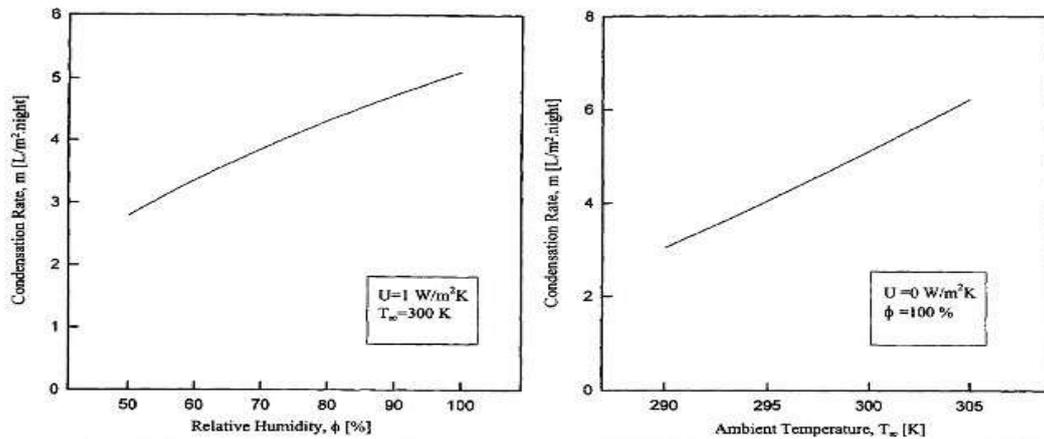
Fig. 3: Effect of relative humidit on condensation rate. Fig. 4: Effect of ambient temperature on condensation rate
