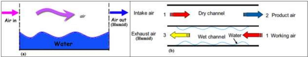
Fig. 1: Schematic element of (a)direct evaporative and (b)indirect evaporative cooling
