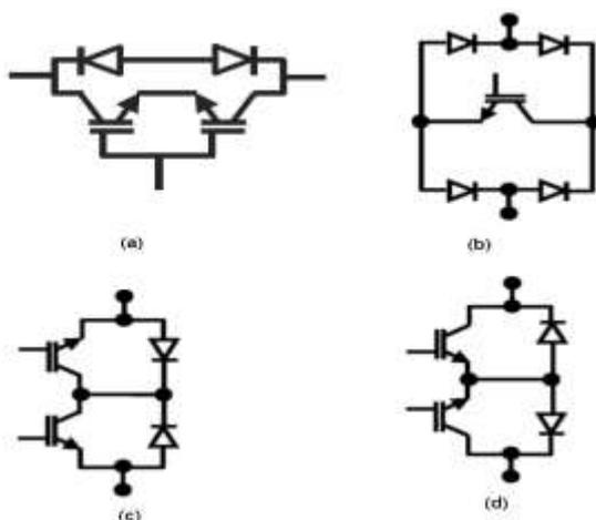
Fig.1: Conventional Bidirectional Switches
