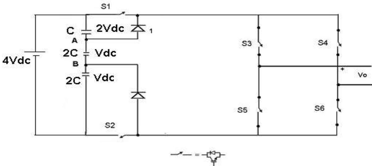
Fig. 6: Proposed Circuit for 9-levels.
