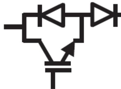
Fig. 2: Unidirectional Switch
