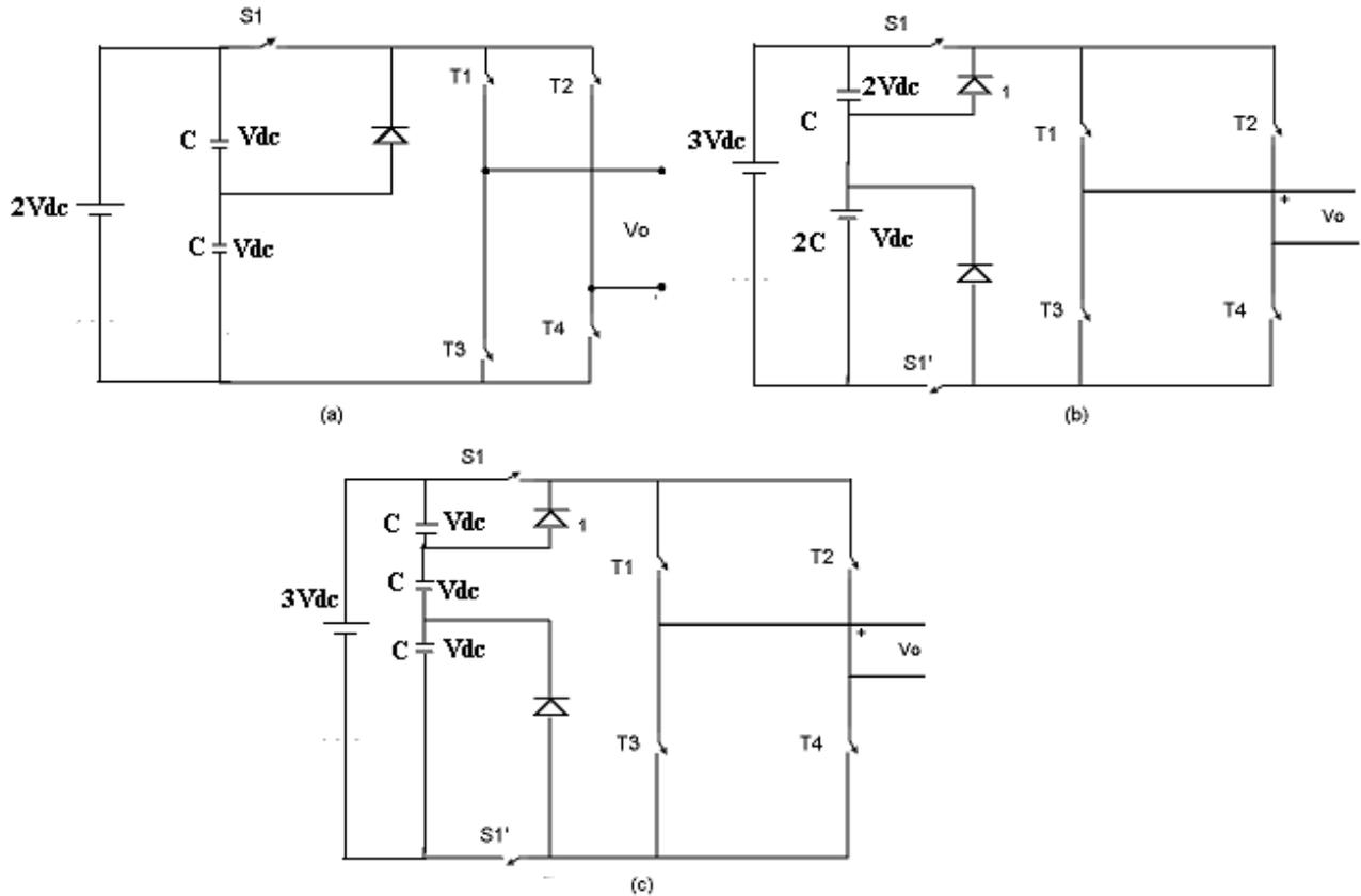
Fig. 4: Single Cell for 5,7 and 7 in (a),(b) and (c) respectively
