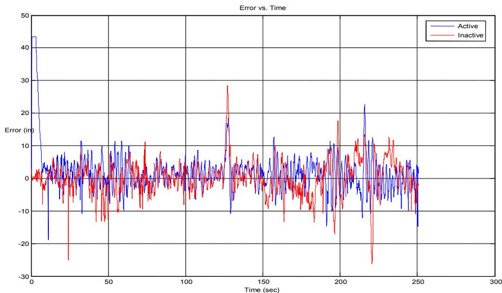
Fig. 7: Height error on Case sprayer at 20 mph with and without fuzzy controller.
