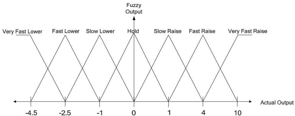
Fig. 5: Membership functions of output.
