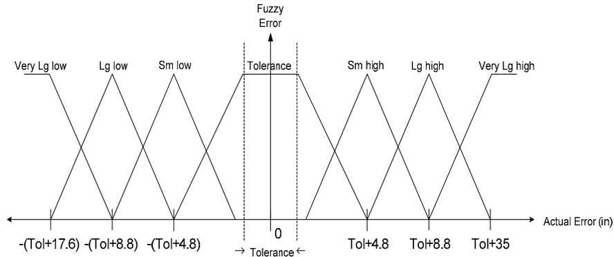
Fig. 3: Membership functions of error.
