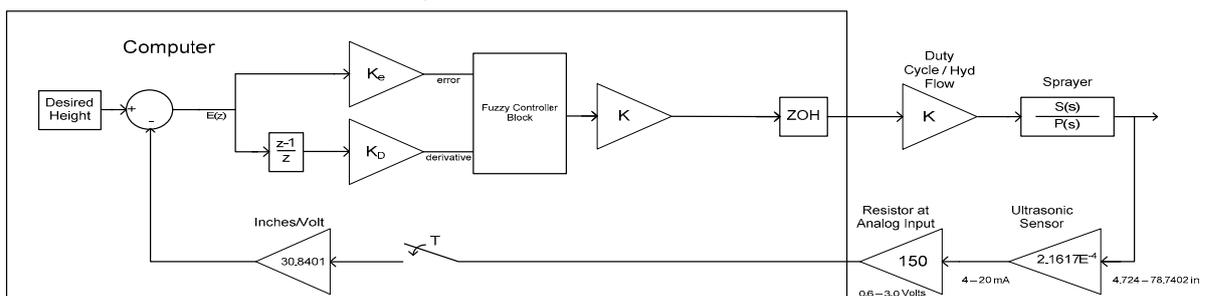
Fig. 2: Block diagram of system with control effort feedback.
