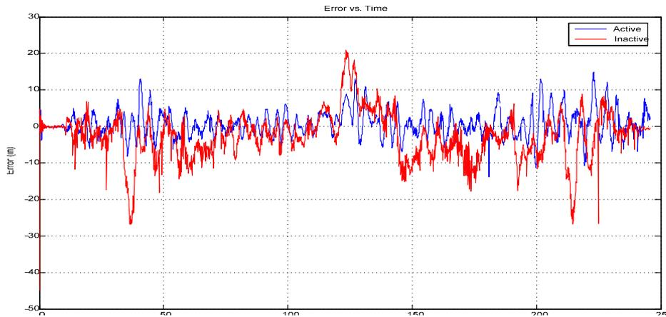
Fig. 6: Height error on Ro-gator sprayer at 20 mph with fuzzy and original controller.
