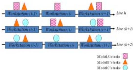
Figure 1. Mixed-model parallel assembly lines
