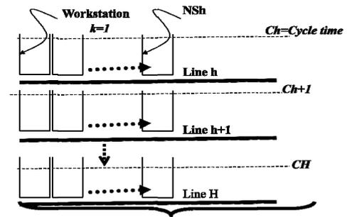
Figure 2. Mixed-model parallel assembly lines balancing problem
