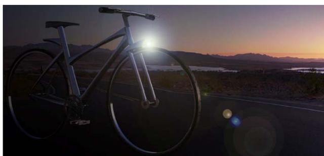
Fig. 7: the integral design of fork and headlight
