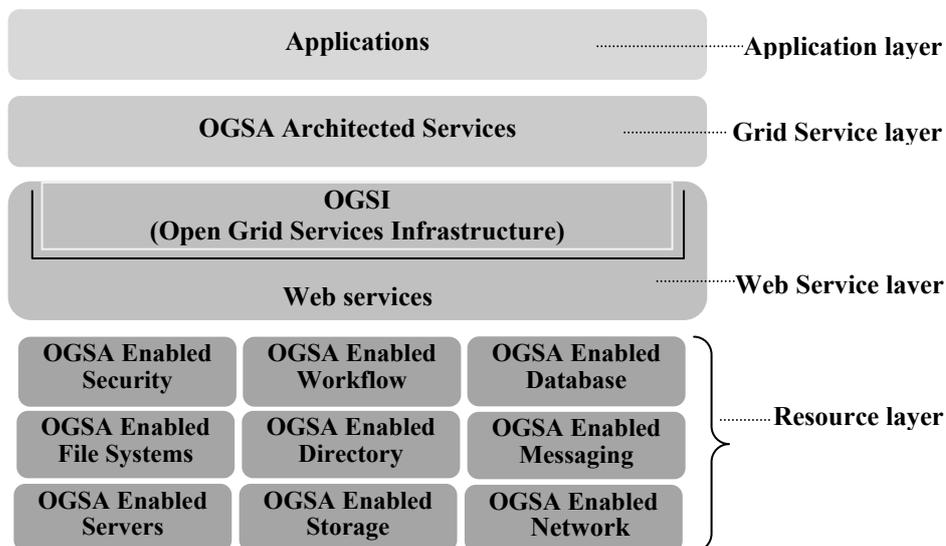
Fig. 1. The structure of Open Grid Services Architecture
