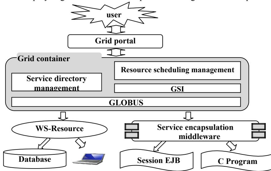
Fig. 3. The working mechanism of SGAP
