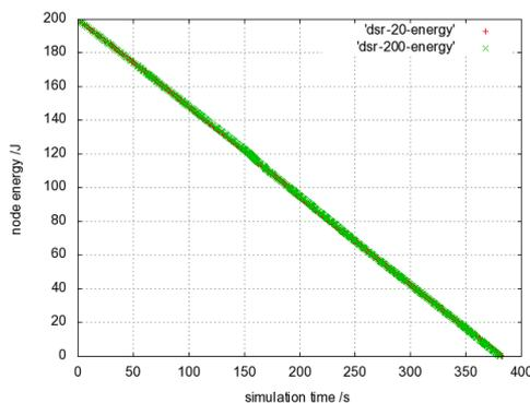
Figure 3. DSR under node density change between 20 and 200 nodes
