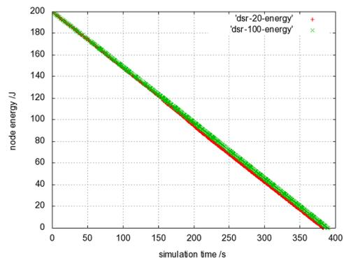
Figure 4. DSR under node density change between 20 and 100 nodes
