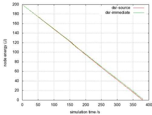
Figure 13. Source node and immediate node energy consumption under DSR.
