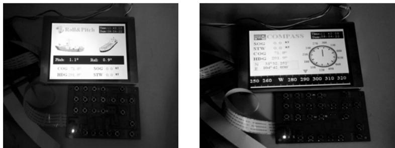
Figure 4 The GUI interface in the satellite compass working process
