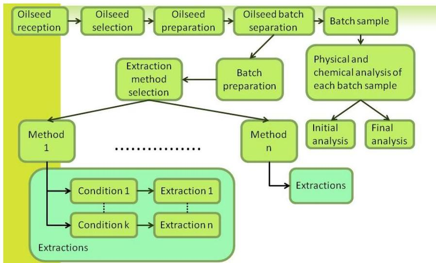
Fig. 2: LAPSDEA's Extraction Experiment Methodology.
