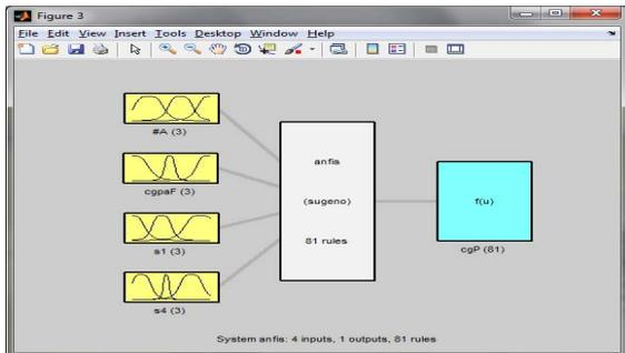
Fig. 4: 4-input 1-output ANFIS architecture model.
