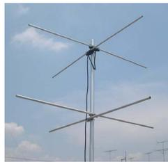
Fig. 3: Crossed-dipole antenna.
