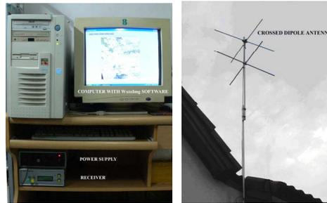
Fig. 6: APT receiving system installation.
