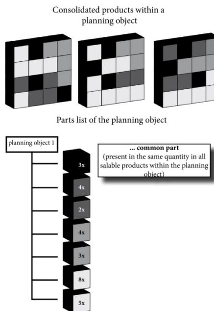
Fig. 4: Parts list of a planning object including a common part
