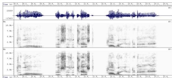
Fig. 5. VaxVOIP Waveform, Wideband and Narrowband spectrograms
