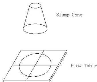
Fig. 1: slump flow test
