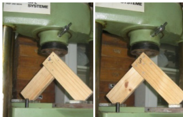
Figure 3. Compressive strength test for the construction fixed with five nails (left) and fixed with five screws (right).
