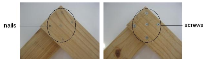
Figure 2. Fixing with five nails (left), fixing with five screws (right).
