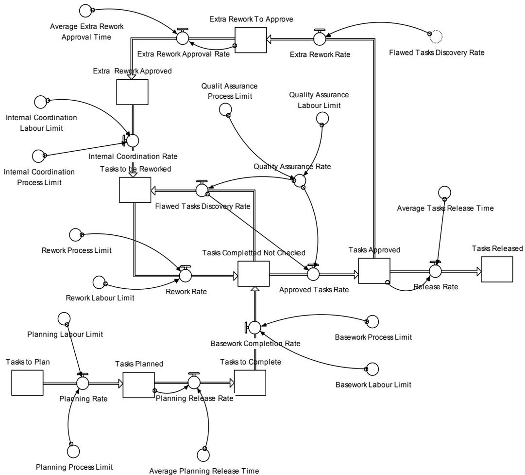
Fig. 1: Evolution of tasks states in the execution process subsystem
