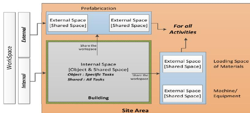
Fig. 2: Configuration of Workspace Allocation Type by Workspace Type.
